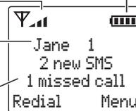
The battery charge level. When this shows 'nearly empty'
